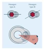
An optimal alignment of the abutment facilitates access to the occlusal screw, which fixes the suprastructure to the abutment. In principle, the abutment should thus have a mesial alignment in the posterior region.
